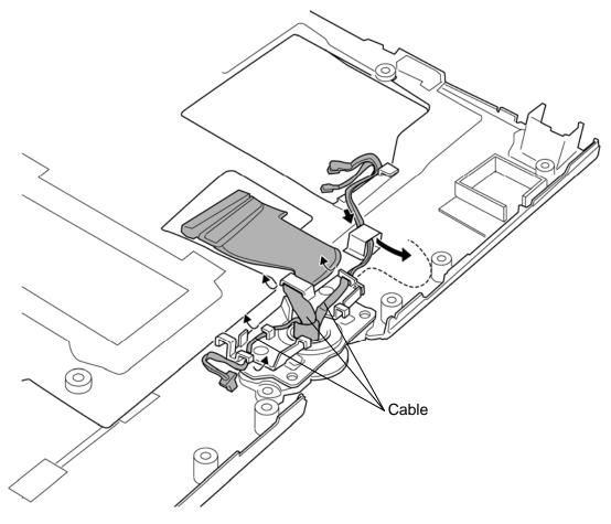
Figure 4-48 Removing the hinge assembly (1)
